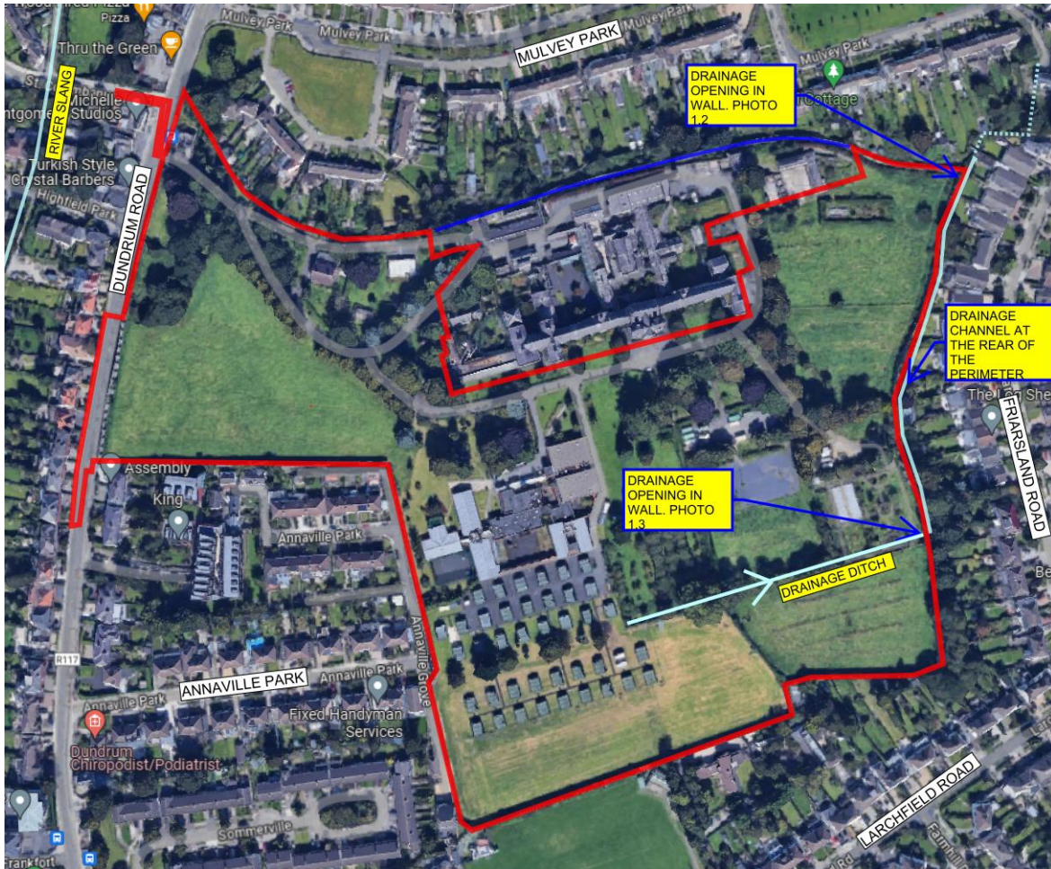
Figure 1.4 Aerial view showing the surface Water drain on the site
