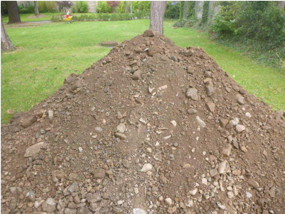
Photo 4.1 Typical Trial Pit Spoil heap (taken from the SI report).
